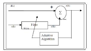
Fig. 1. General setup of adaptive filter.
