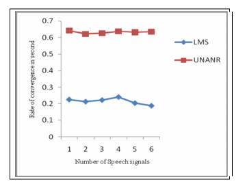
Fig. 6. Plot of Rate of convergence versus to different samples of speech signal.
