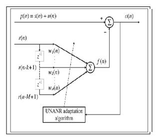
Fig. 3. Detailed structure of the UNANR model.
