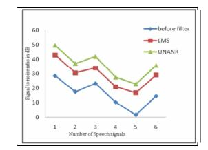
Fig. 4. Plot of SNR (dB) before filtering process, System's improvement with respect to LMS filter and UNANR model versus to different samples of speech signal.
