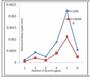
Fig. 5. Plot of estimated root mean square error (RMSE) versus to different samples of speech signal.
